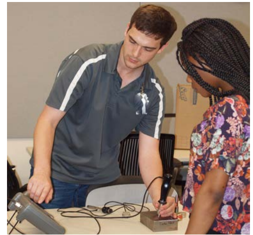
Josh Dean (E06), left, an Engineering apprentice on rotation to Dept. O31, demonstrates a portable hardness test to a student at The Apprentice School July 15. Photo by Nicole Lawrence (O31)
