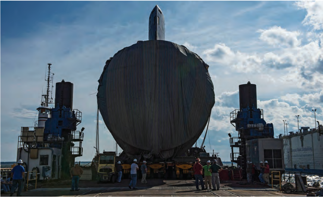
View September's edition of "Hot Shots" on Yardnet . Pictured on left: The bow section of the Virginia -class submarine Colorado (SSN 788) is loaded onto the sea shuttle for its journey to Electric Boat. Photo by John Whalen ; Pictured on right: Shipbuilder Jessica Brown keeps her eye on the task at hand while sewing material in the Sail Loft. Photo by Ricky Thompson
