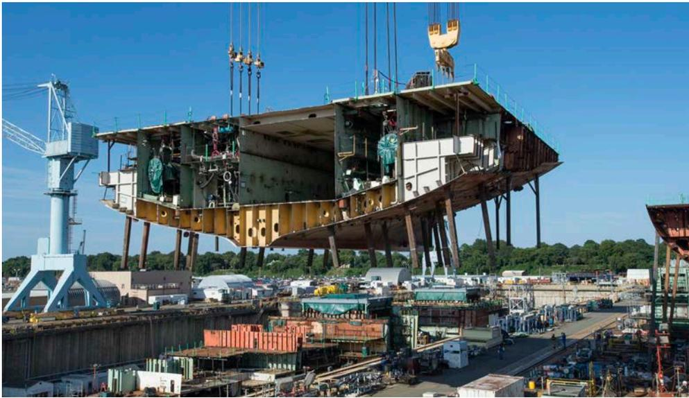
NNS placed a 900-ton superlift into dry dock, continuing construction of the nuclear-powered aircraft carrier *John F. Kennedy* (CVN 79). Photo by **John Whalen**
