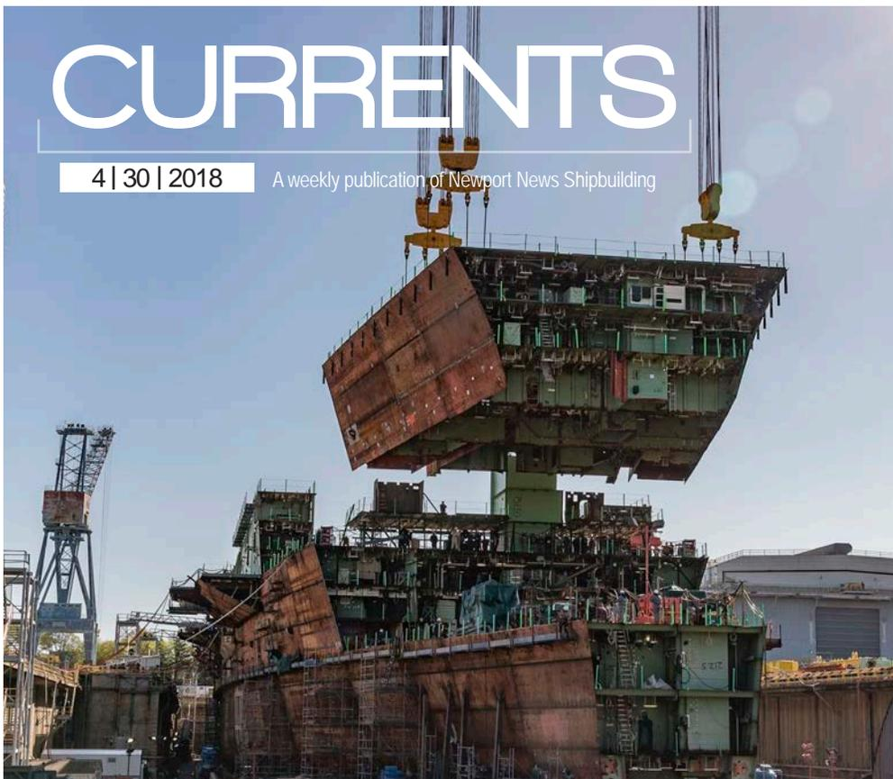
Shipbuilders install a 750-metric-ton forward section of *Kennedy's* main deck. Photo by John Whalen
